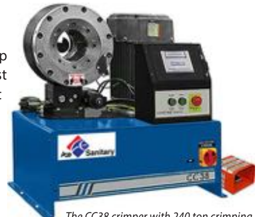
The CC38 crimper with 240 ton crimping force has the capacity to crimp 1 1/4" multi spiral hydraulic hose and 2" industrial hose.
